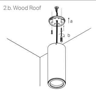
Ensure wood thickness is not less than 5mm!
