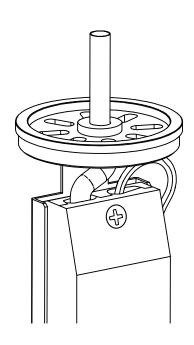
Cover the installation cables with the cable protector and lock the cable of the luminaire with the driver cover.
