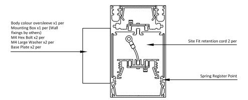
LED Tray & Driver connection polarity must be kept RED to RED & BLACK to BLACK Retention cords must also be connected to body via M4x6 Pan Pozi screws
